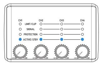
Active Mode is indicated by a Blue LED, the amplifier is connected to power and ready to pass signal.
