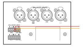
Unbalanced Link Wiring
