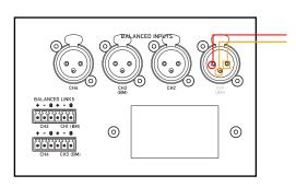
Unbalanced Input Wiring
