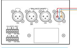
Bridged-Mono Balanced Input Wiring
