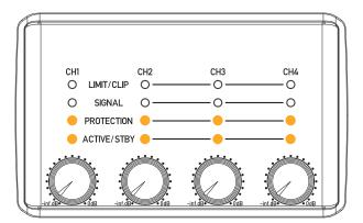
The Orange LED's indicates the amplifier is in Standby, a power saving mode. This mode can be enabled by toggling the under panel A-STBY switch from Off to On. In this mode if no signal is detected for 25 mins the amplifier will "sleep" and wake within 660ms of detection of signal.
