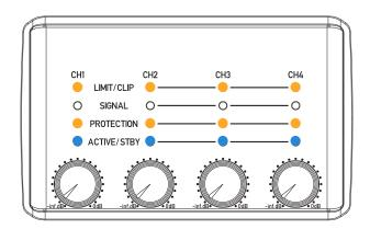
Mute mode puts the amp into a "light sleep" and occurs when the Standby option has been selected and no signal has been detected for 10mins, if the amplifier detects signal it will wake within 1ms. When no signal has been detected for 25 mins full sleep mode will activate.
