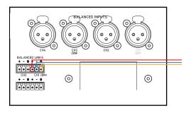
Balanced Link Wiring
