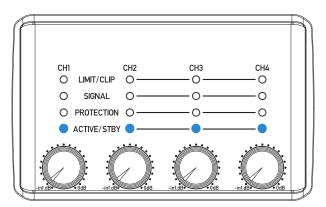
Active Mode is indicated by a Blue LED, the amplifier is connected to power and ready to pass signal.
