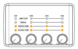
The Orange LED's indicates the amplifier is in Standby, a power saving mode. This mode can be enabled by toggling the under panel A-STBY switch from Off to On. In this mode if no signal is detected for 25 mins the amplifier will "sleep" and wake within 660ms of detection of signal.
