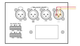
Unbalanced Input Wiring
