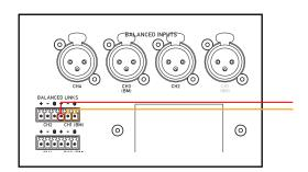
Unbalanced Link Wiring
